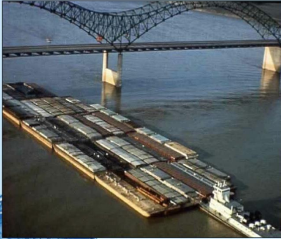
Large mixed tows of over 30 barges are common on open water stretches of the Lower Mississippi River "Setting the course"
