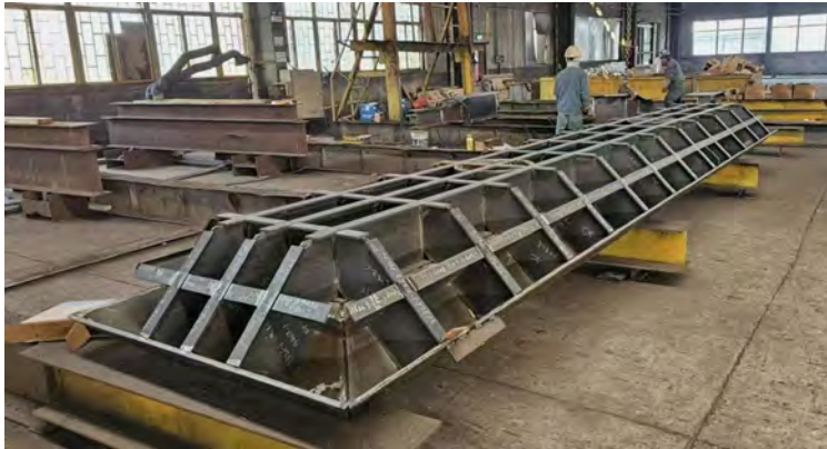
Figure 9.2: Typical fender panel cross section samples (U profile on left, T-profiles on right side)
