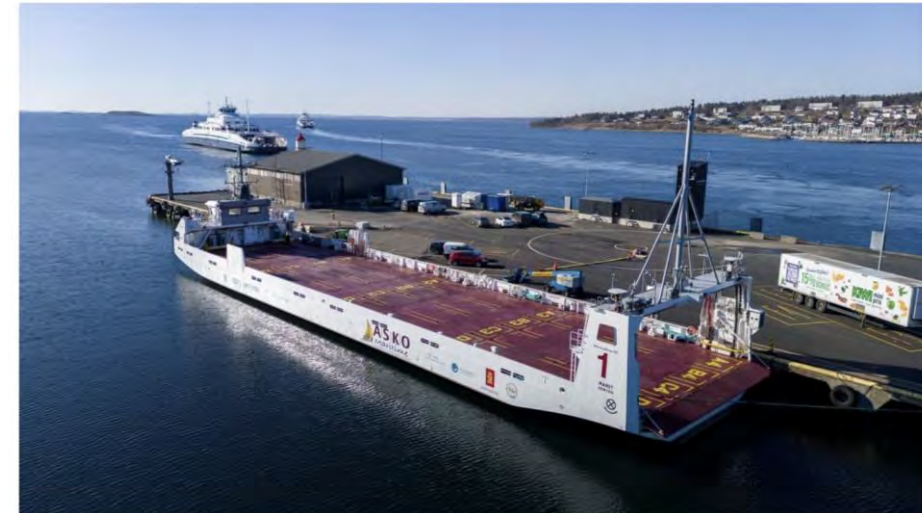
Battery-powered ASKO barge. Courtesy of Kongsberg.
