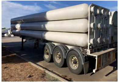
Compressed hydrogen MEGCs have up to 400 cylinders and Tube trailers typically have 8 to 10 tubes.
